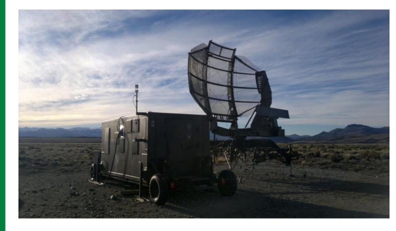
The MTPS-43 is the result of the Invap Radar Modernization Process (IRMP) over the old Westinghouse TPS-43 Tactical Air Defence 3D Radar. This equipment upgrade has proven to be successful in meeting the proposed objectives:
