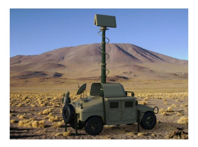
RMF-200V is a multi-mission / multifunction 3D short range air defence radar featuring a lightweight compact design based on state-of-the-art technology. With a detection range of up to 200km
